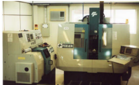
(b) the CNC lathe and the CNC mill (both made by Feeler)
